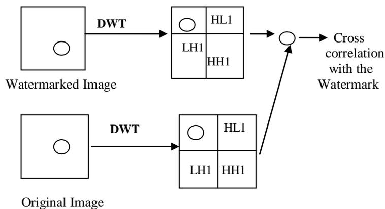
Fig. 2 Decoding of original and watermarked image
