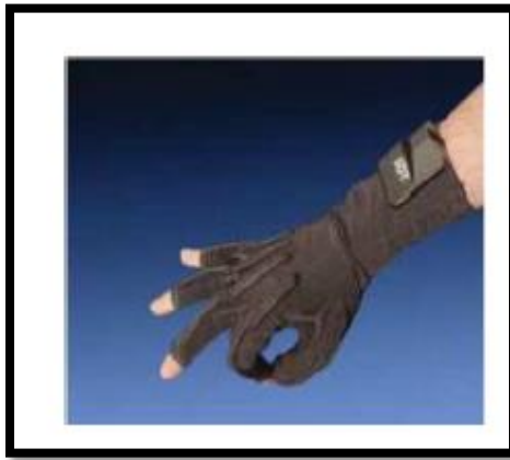
Fig.2 Instrumented /Data Glove
