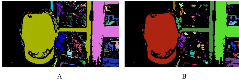
Fig. 6: Illustration of erosion (A) face segment before erosion (B) Face segment after erosion
