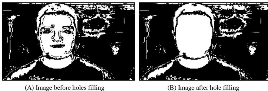
Fig. 7: Example of a hole filled image
