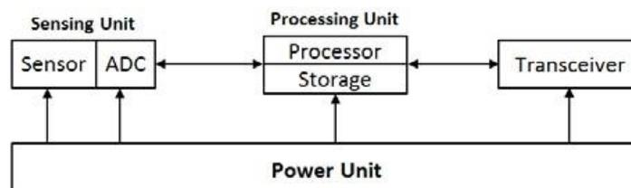
Figure 1. Typical sensor node architecture
