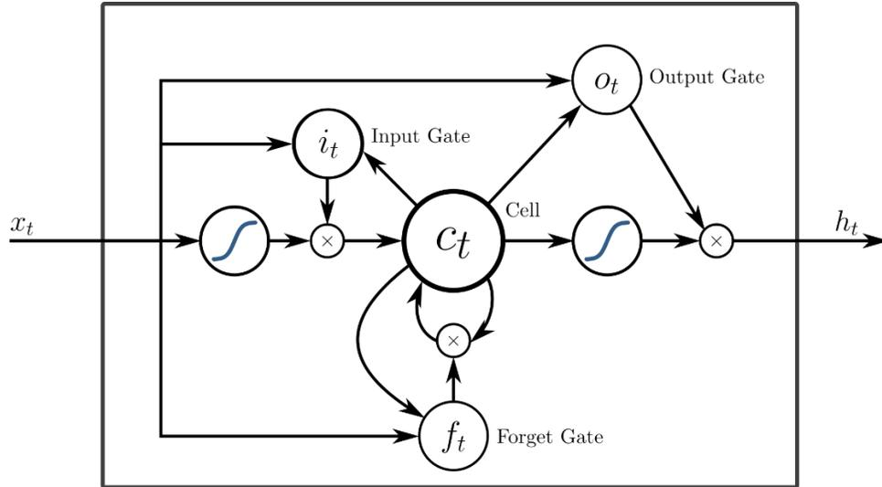
Figure 2: Illustration of an LSTM block.
