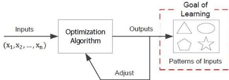
**Figure 6:** Mechanism of unsupervised machine learning algorithms [8].
