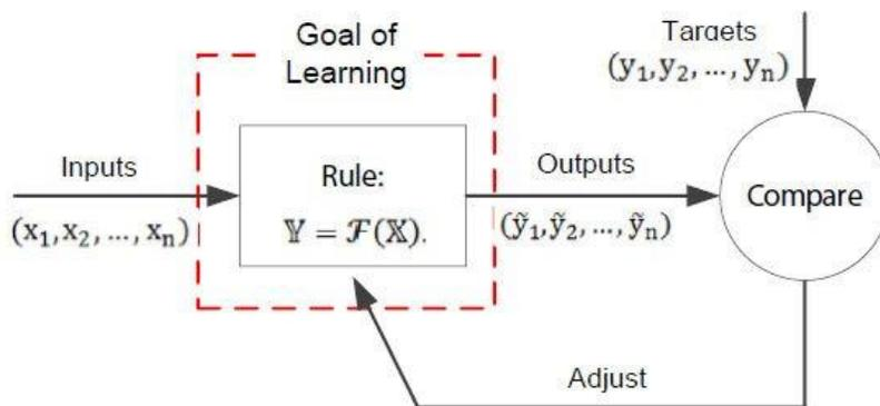
**Figure 5:** Mechanism of supervised machine learning algorithms [8].
