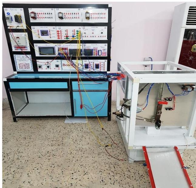
Figure 10: the practical connection of smart factory using PLC and NodeMcu
