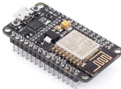
Figure 1.4: the NODEMCU 8266 board
