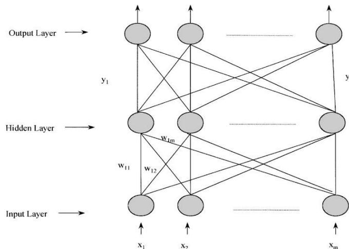
Fig 2.2.1 Architecture of Neural Network
