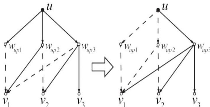
Fig. 1. Illustration of the pruning procedure in ConMap without receiving energy. The left part denotes a subgraph of a constructed Steiner tree that is not in canonical form. The right part represents the corresponding subgraph after the pruning procedure: absorb the original vertices that are connected to  $w_{up2}$  into  $w_{up3}$ . And the solid lines are the way that we have chosen to transmit and the dashed lines present the way that we have not chosen.
