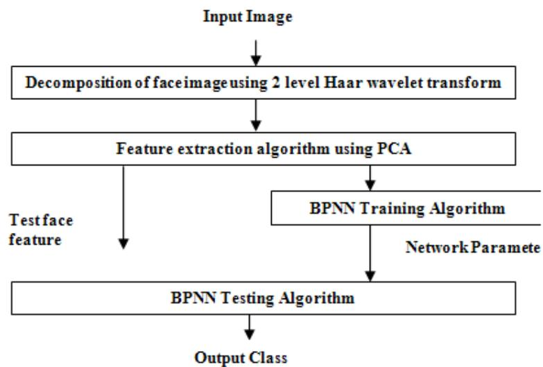
Fig. 6 Flow diagram of Proposed Face Recognition System
