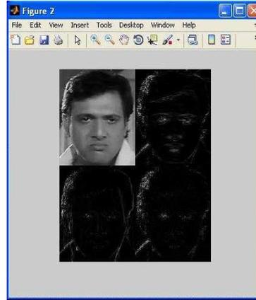
Fig. 8 Decomposed Image using Haar Wavelet Transform
