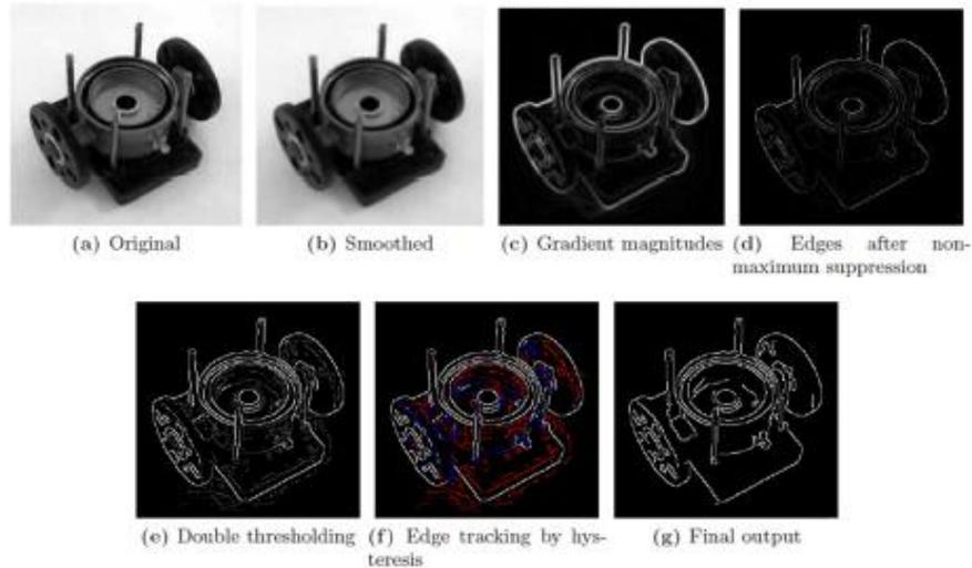
**Figure 3: All steps of the edge detection.**
