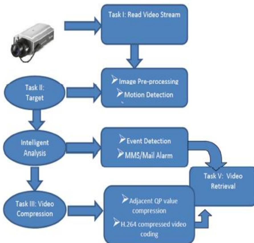
Fig 1: Intelligent Video Surveillance System Framework
