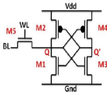
Fig 3. Five Transistor (Single Ended ) SRAM Cell
