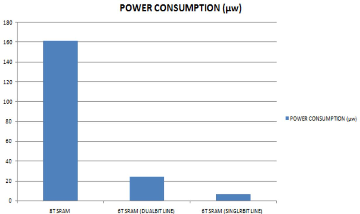
Fig 8 Comparison of power for various SRAMs
