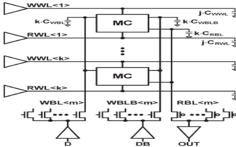
Fig.4 Bit line structure of the SRAM sub array
