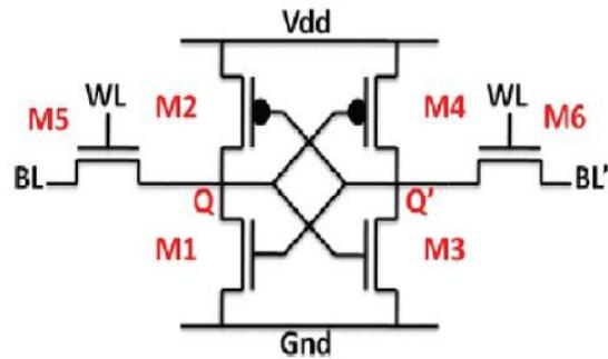
Fig 2. 6 transistor standard SRAM Cell
