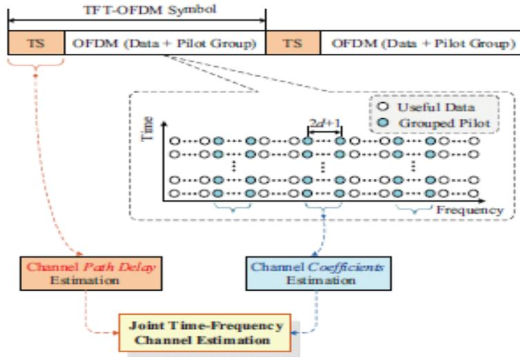
Fig. 3: Signal structure and the corresponding joint time-frequency channel estimation of the TFT-OFDM scheme [1]
