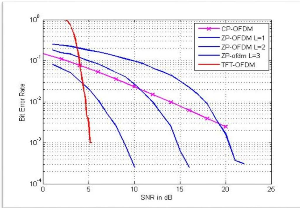
Fig.4. BER performance comparison between the proposed TFT-OFDM scheme and the traditional schemes
