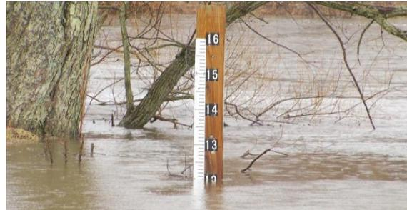
The level of water is measure with the help of that scale is it normal, low or danger. According to the situations the flow of water is controls with the help of Dam’s gates. Here we want to use the Switch as the water measure scale and intelligent device that is capable of sends acknowledgement signal to the source end to control the transfer rate as per need.
