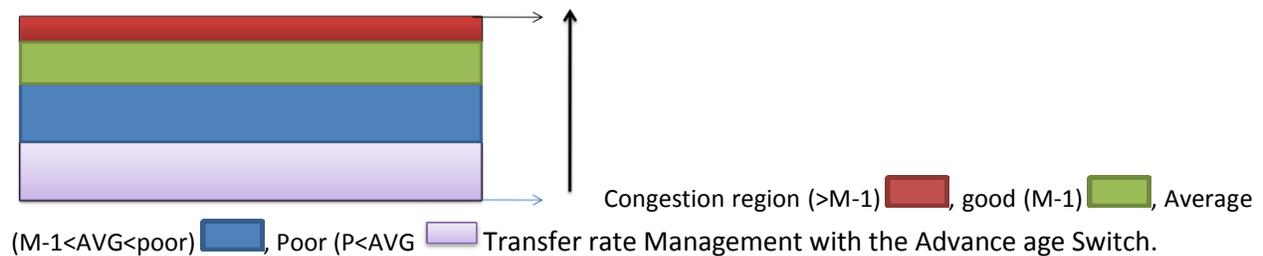
When the transfer rate is below the good strength then it will sends a signal to the source end to increase the rate of data transmissions. On the another hand as it encounter the transfer rate of data is higher than the good sign then it will send another signal to source end to reduce the rate of data transmission to keep the error and congestion free data transmission. This will helps us to setup an intelligent control on the interconnecting devices or media to perform better.
