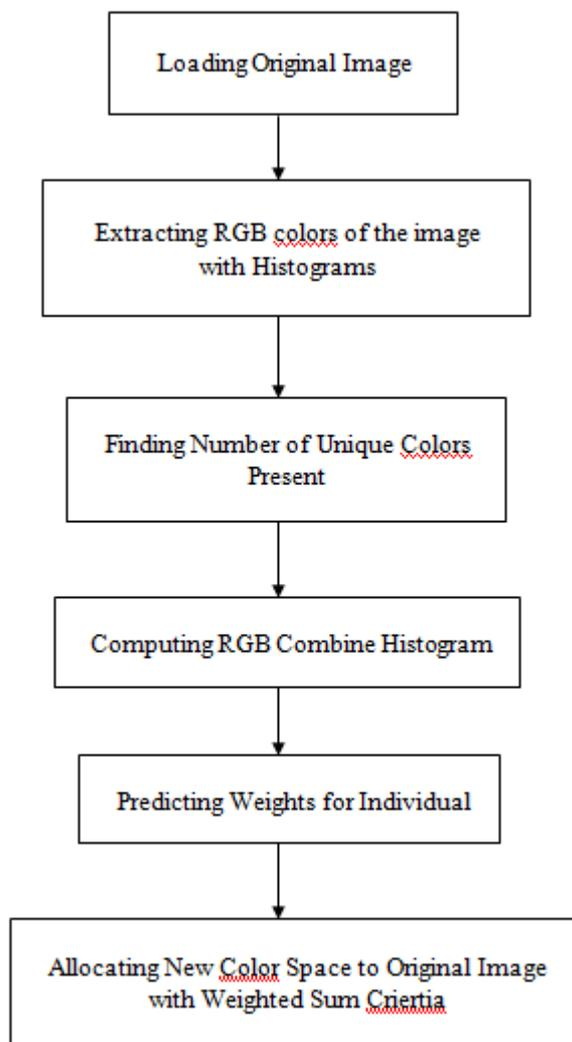
Fig 2: Block Diagram of the Proposed Algorithm
