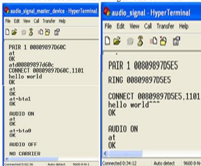
Fig. 8 Results of audio/voice transfer between transmitter (left side) and receiver (right side) units on windows hyper terminal.
