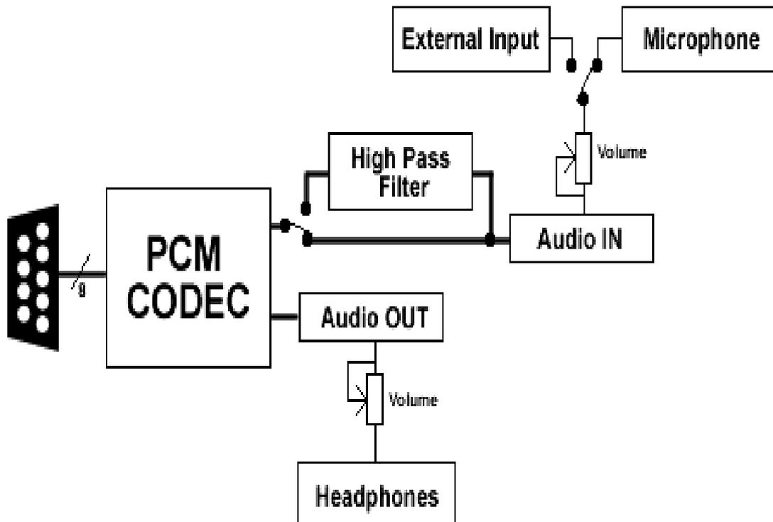
Fig. 2 Block schematic of audio codec board [3]
