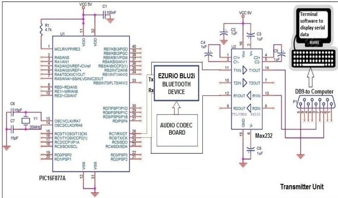
Fig. 4 System integration of transmitter unit
