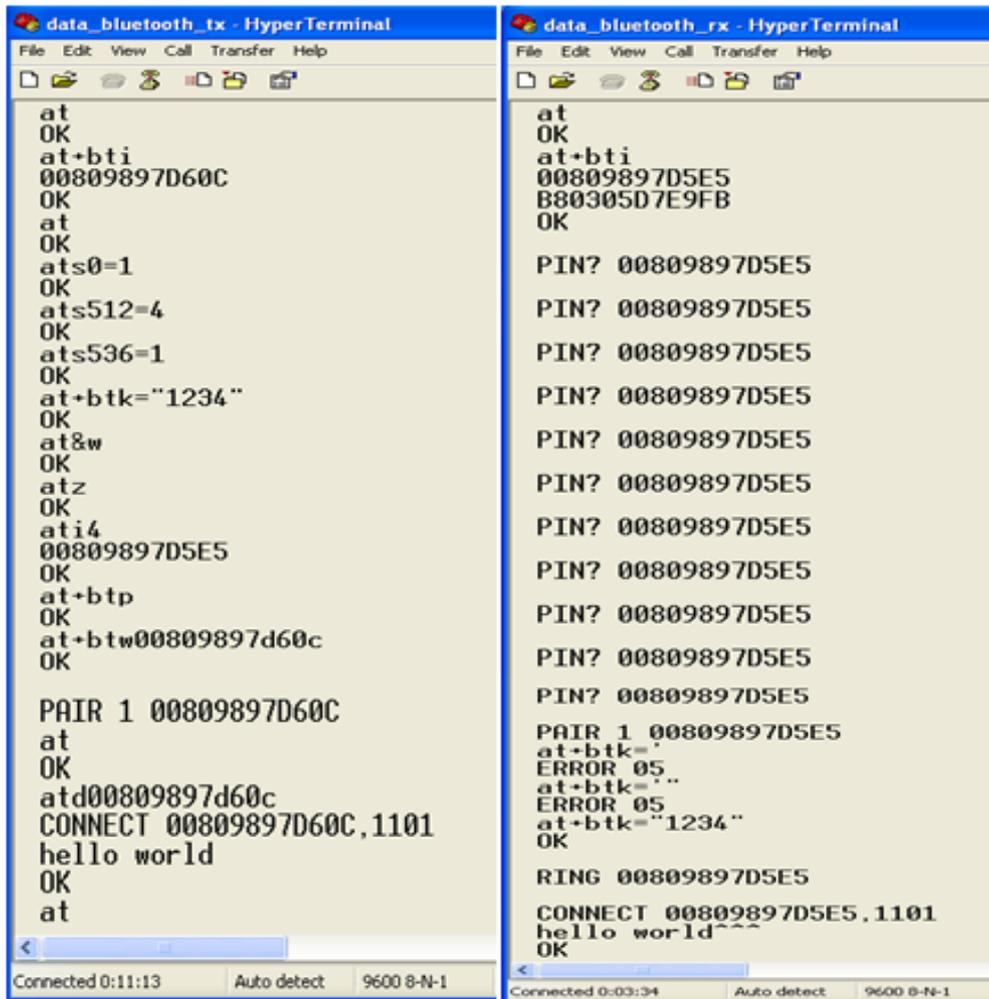
Fig. 7 Results of real time data transfer between transmitter (left side) and receiver (right side) units on windows hyper terminal.
