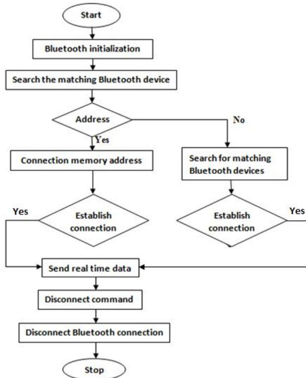
Fig. 6 basic design flow chart of Bluetooth device
