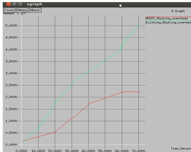
**Graph 3:** Comparison of Routing Overhead between Existing and Proposed MCQ-TC
