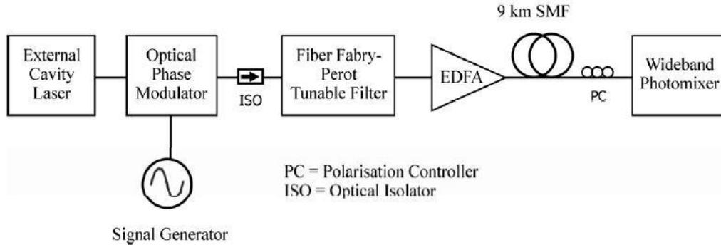
**Figure 4 Remote Heterodyning by Using a Filter.**
