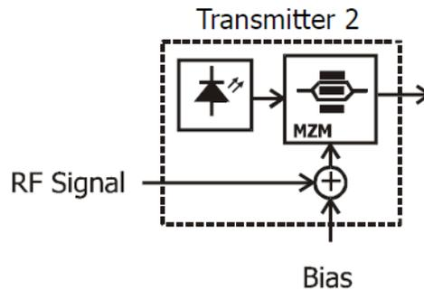
**Figure 3 DIM Method By External Modulator**
