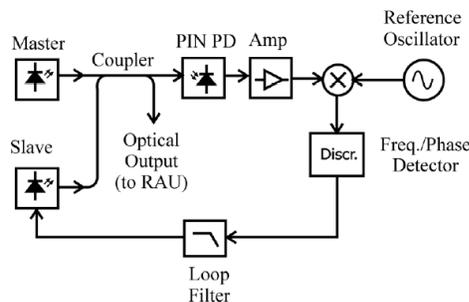
**Figure 5 Principle of Optical Frequency-/Phase-Locked Loop**
