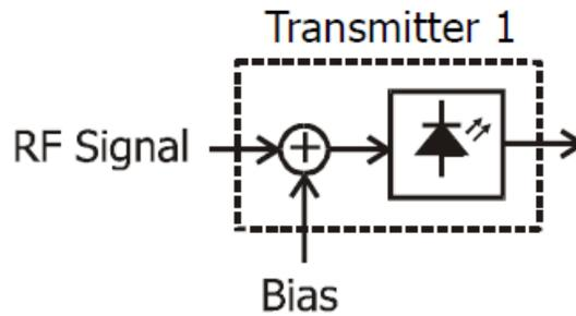
**Figure 2 Direct Intensity Modulation Method By laser.**
