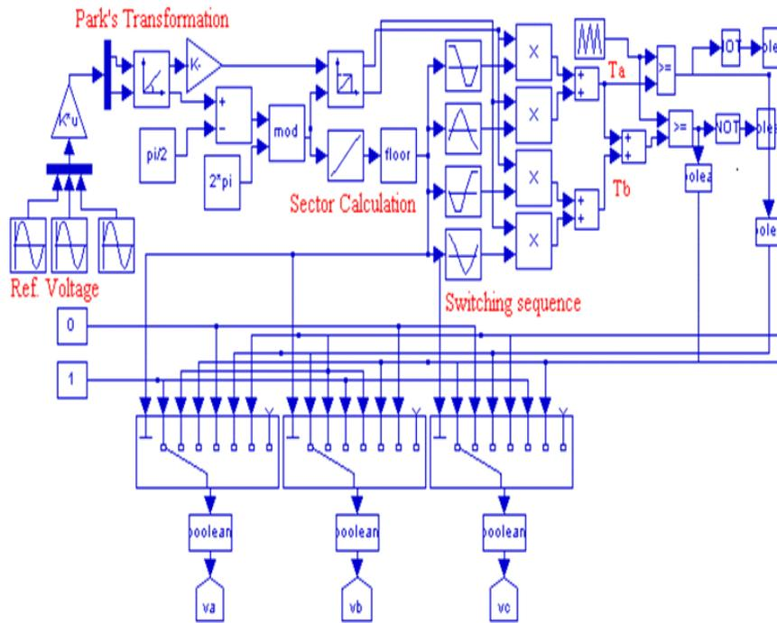
Figure.3 represents simulink model of SVPWM
