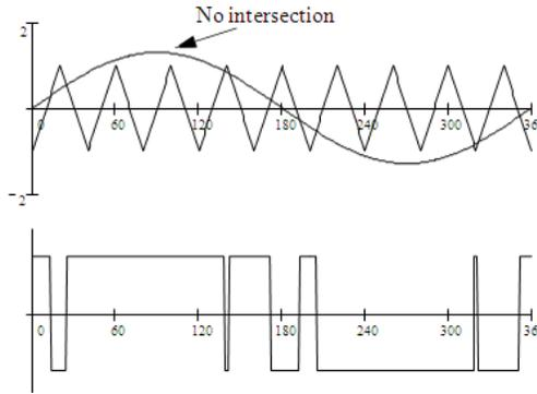
Figure.1 represents sampling of modulation wave with a triangular wave.
