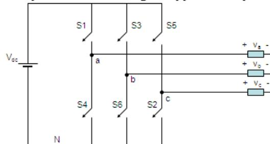
Figure.5 represents a voltage source inverter
