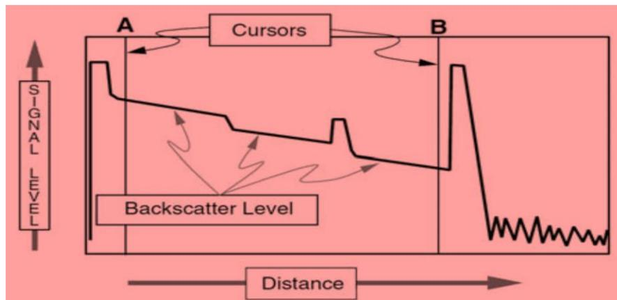
Figure 2: Components of OTDR Trace Display
