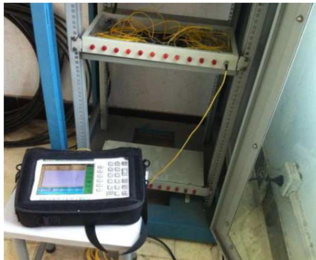
Figure 3: OTDR connected to fiber under test
