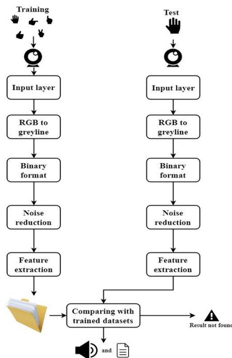
Figure 1: Architecture Diagram for Gesture Recognition System
