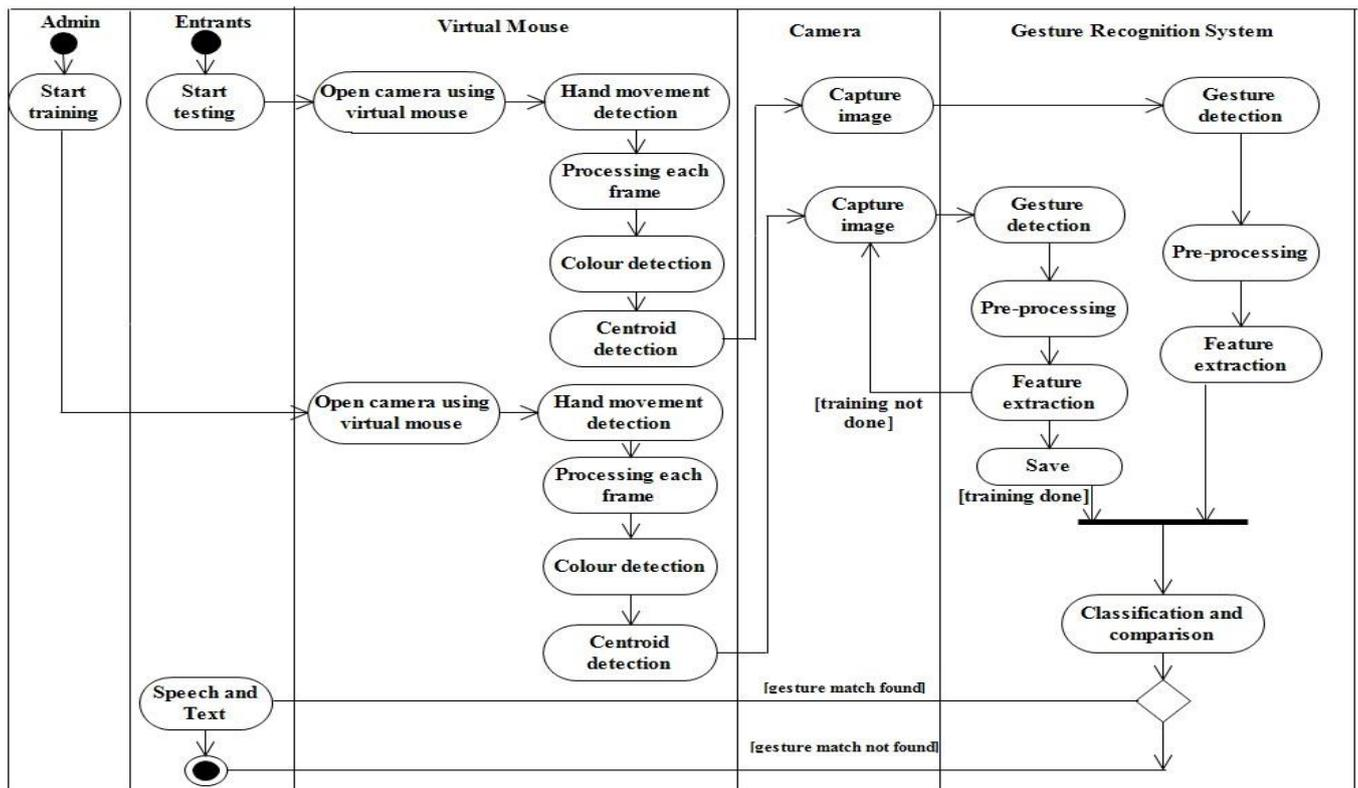
Figure 2: Activity Diagram for Gesture Recognition System
