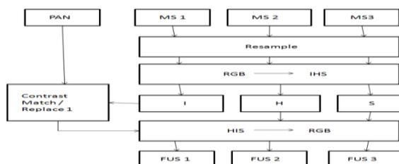
Figure 3: Block scheme of the IHS fusion method
