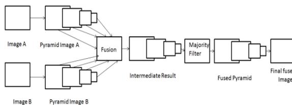
Figure 5: Block scheme of the Laplacian Pyramid fusion method
