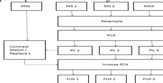
Figure 4: Block scheme of the PCA fusion method
