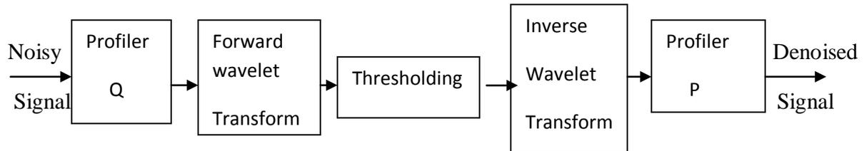
Figure1: Diagram of wavelet based image De-noising
