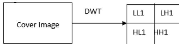
Fig. 2 one level of Wavelet Decomposition
