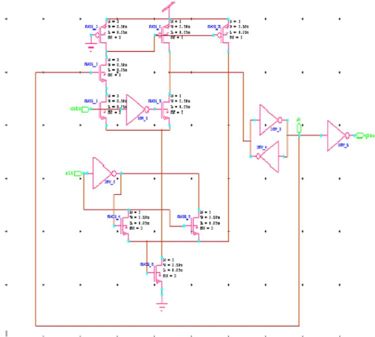
Fig 4: conditional pulse enhancement scheme
