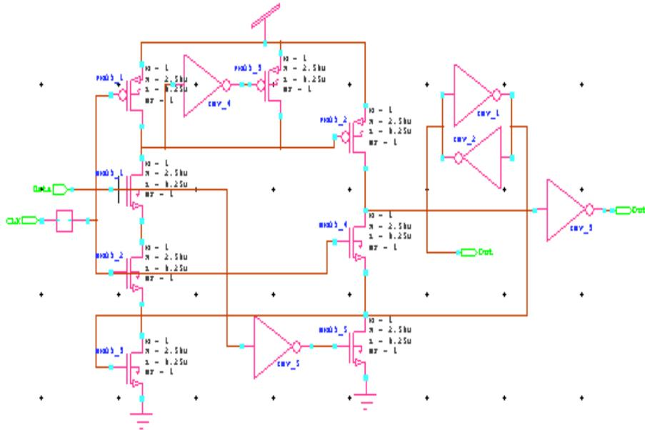
Fig: 2 conditional discharge flip-flop
