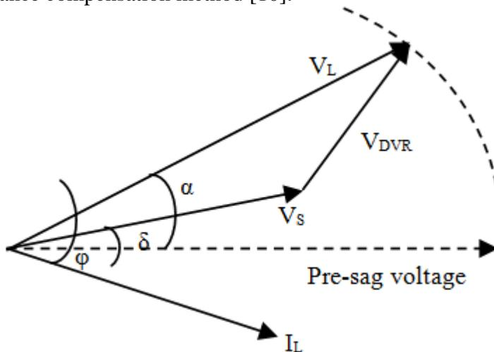
Figure 4. In-phase advance compensation method
