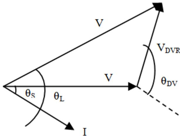
Figure 2. Pre-fault compensation method.
