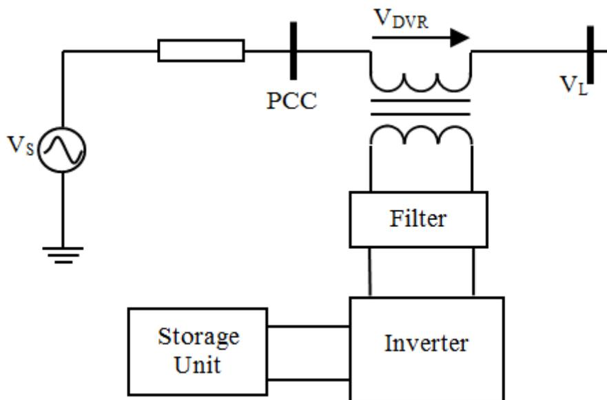
Figure 1. Basic structure of DVR
