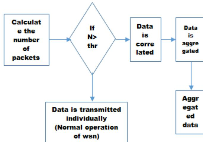
Fig4: Node-level data aggregation and correlation
