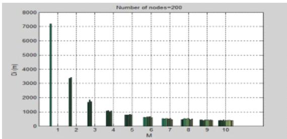
**Figure3.** Comparison of path distance under different partition number.
