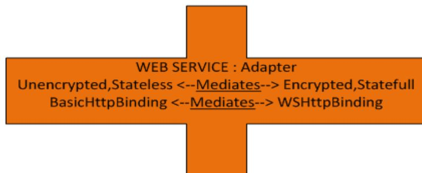
Figure adapter as a mediator between different protocols and data transmissions
