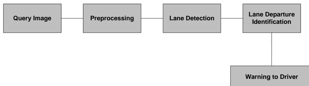
**Figure 1.5 Graphical representation of lane departure warning system**
