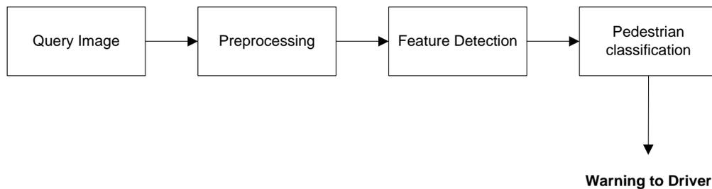
**Figure 1.4: Graphical representation of pedestrian detection system**
