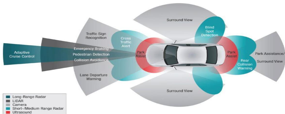
Figure 1.1: Various features of typical ADAS
