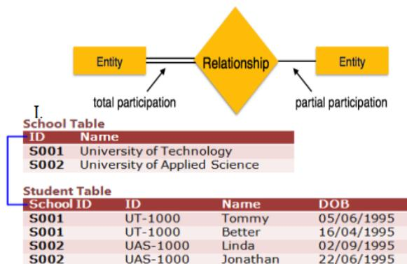
Figure 2.4: Entity Relationship Diagram of the existing system [4].
