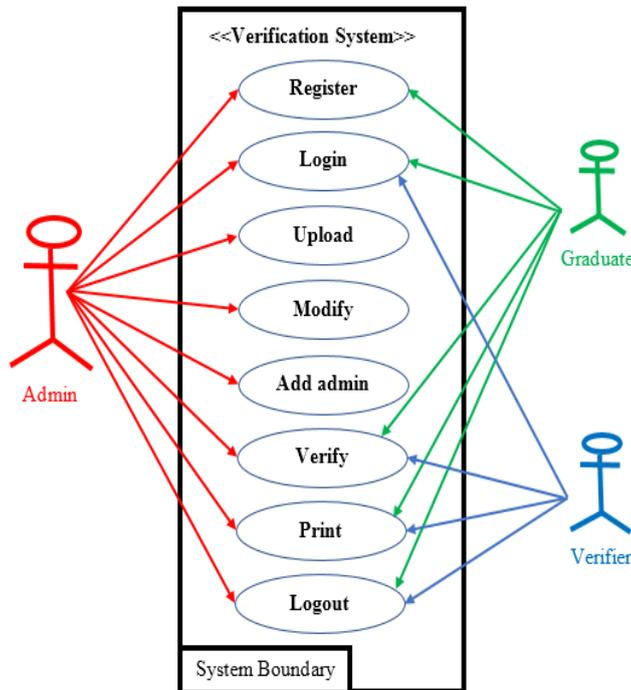
Figure 4.5 the proposed system use case diagram.
