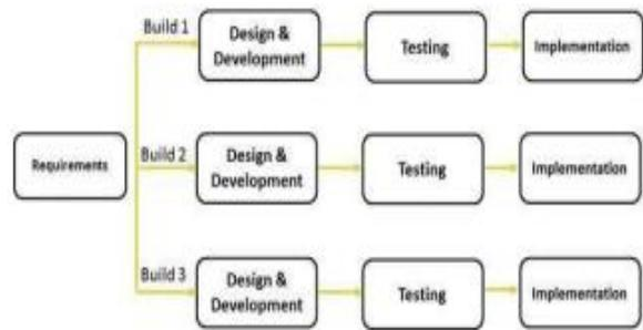
Figure 4.2 Typical Iterative model diagram [4].
