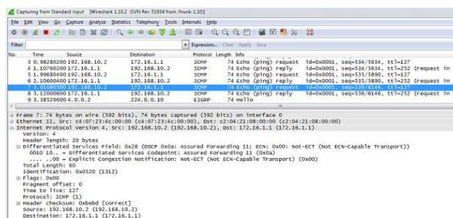
Fig. 9 ICMP packet details before reaching Core network at ISP-1 router
