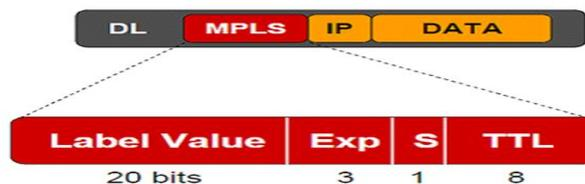
Fig. 3 MPLS Shim Header
