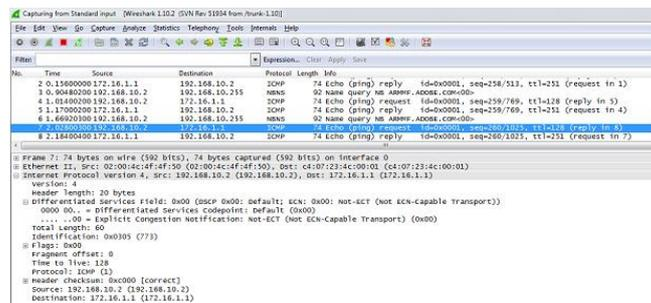
Fig. 8 ICMP packet details before reaching CE-1 Router
