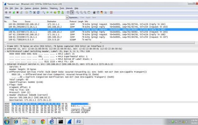
Fig. 10 ICMP packet details through MPLS network
