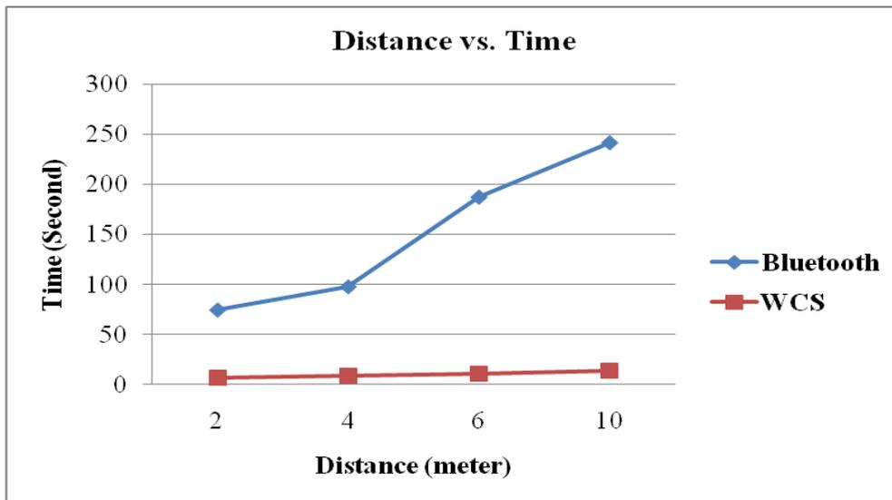
Fig. 3 Bluetooth vs. WCS file transmission speed
