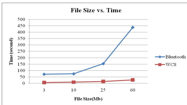
Figure 9.8 Bluetooth vs. WCS performance for varying file size
