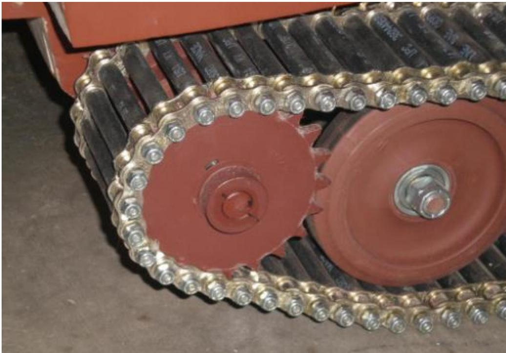
Fig. 2 Robotics Construction showing Mechanical Aspects
