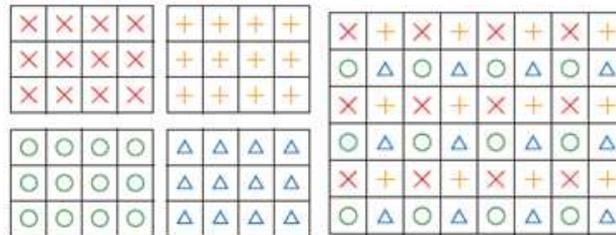
Figure-1.1:-Ideal super-resolution setup. Four images are taken with relative shifts of half a pixel in horizontal, vertical, and diagonal directions (left). Their pixels can then be interleaved to generate a double resolution image (right) [3].
