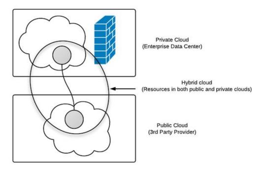
Figure 2 - Cloud Deployment Model
