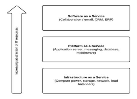
Figure 3 – Levels of abstraction in cloud computing service models
