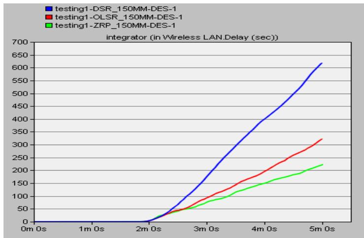
Figure 5: Wireless LAN Delay (nodes=150)
