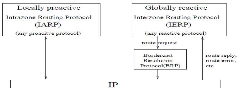
Figure 3. The different component of Zone Routing Protocol
