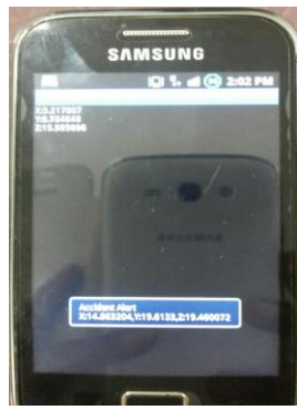
Fig.4: Snapshot showing the reading of accelerometer
