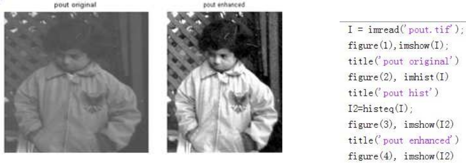
Figure (2): Shows pout image before and after contrast enhancement
