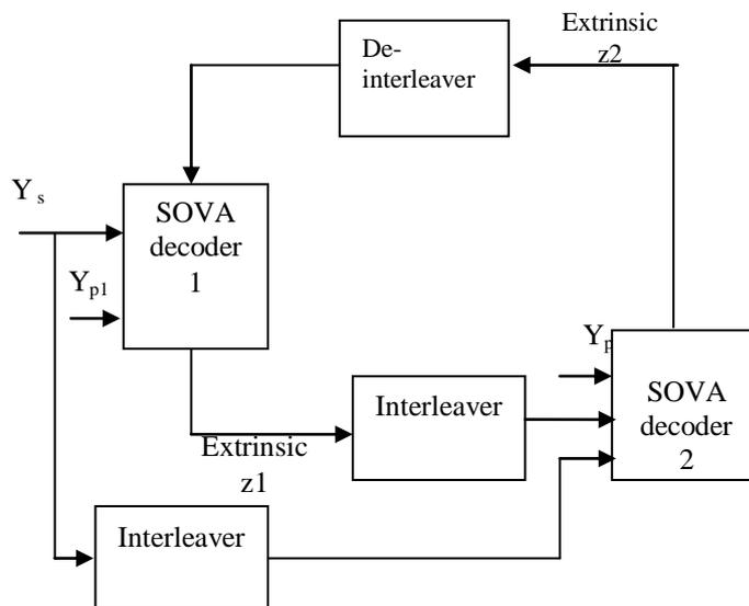
Fig.3 Turbo decoder
