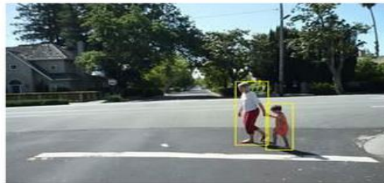
Fig. 5. Detection of Pedestrian using HOG
