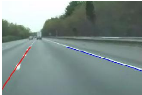
Fig. 8. Detection of lane markings using Improved Hough Transform
