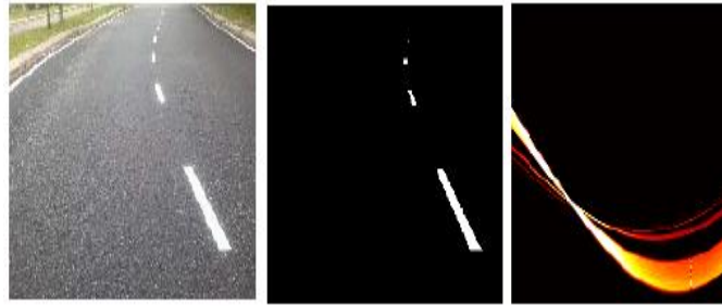
Fig. 1.Original image, Process image and Hough Transform image
