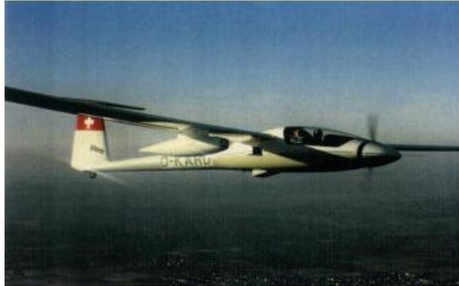
Figure 1: Stemme motorglider with pod under win
