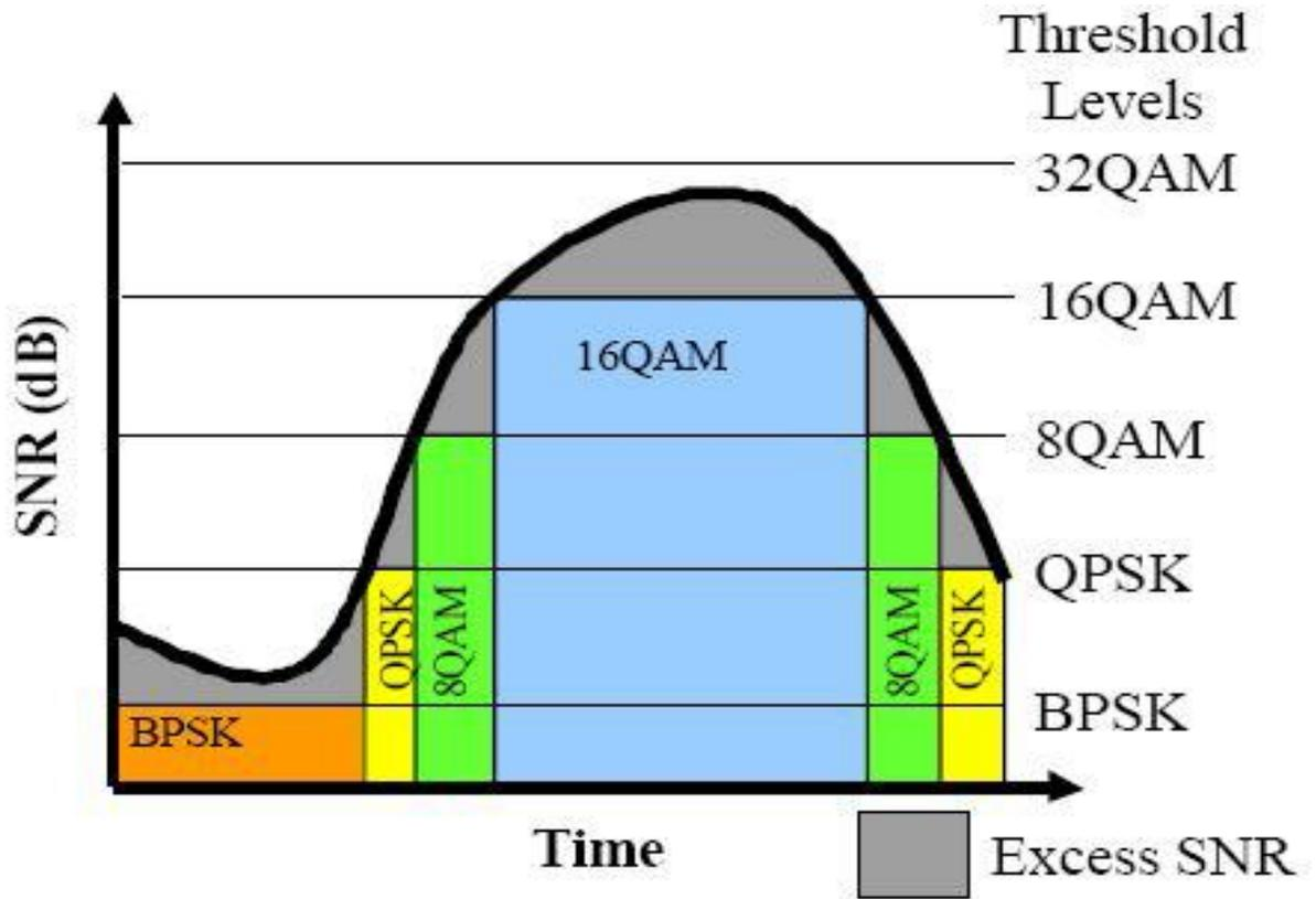
Figure 3:-Assignment of Modulation Scheme Based on SNR
