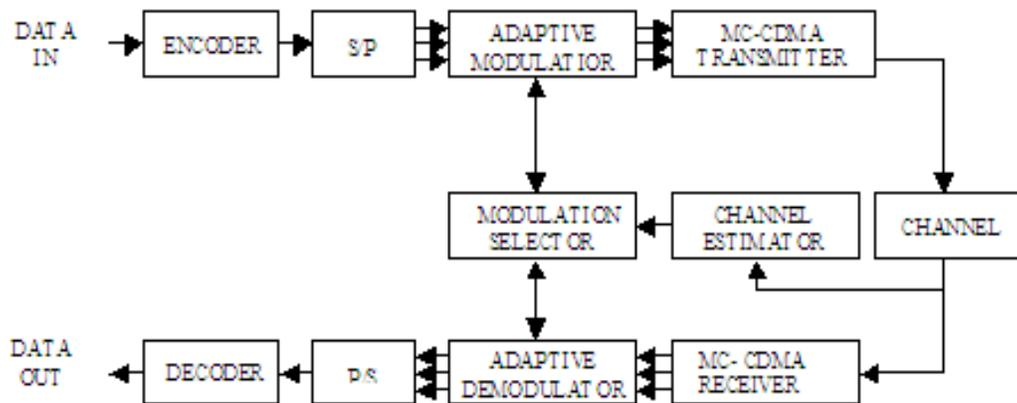
Figure 2 :-Proposed System Model for Adaptive Modulation based MC-CDMA system
