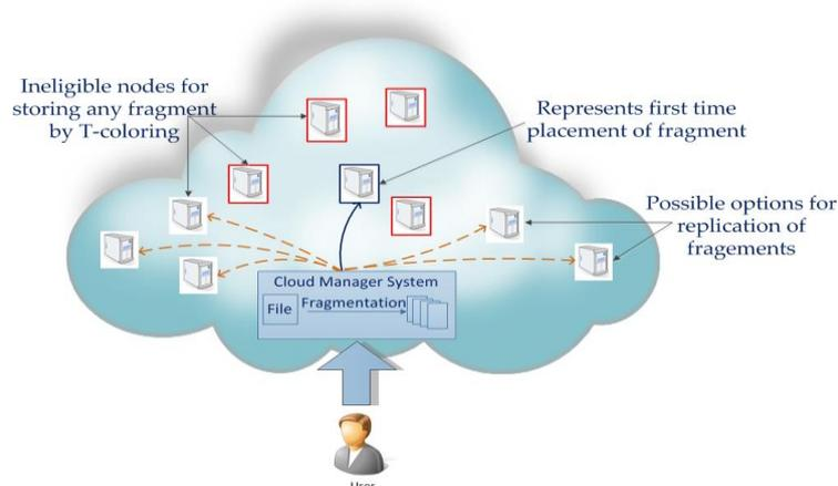
Figure1- Data Slicing and Replication Methodology
