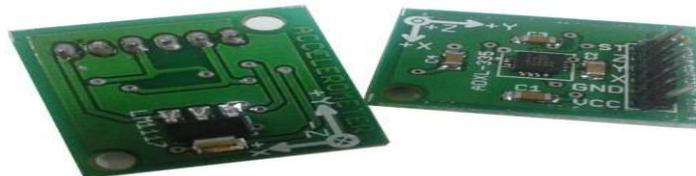
Figure: MEMS Sensor
