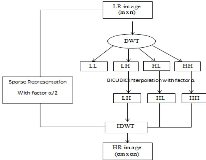
**Fig. 1. DWT and Sparse based super resolution**
