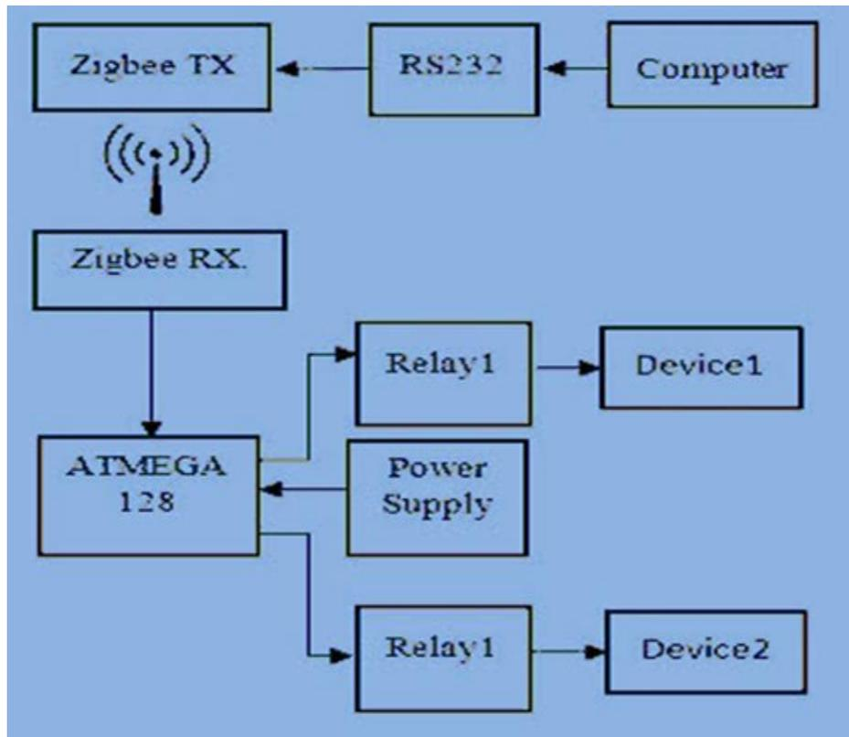
Fig. 2 Block diagram of Enabling Mobile Devices For Home Automation Using Zigbee
