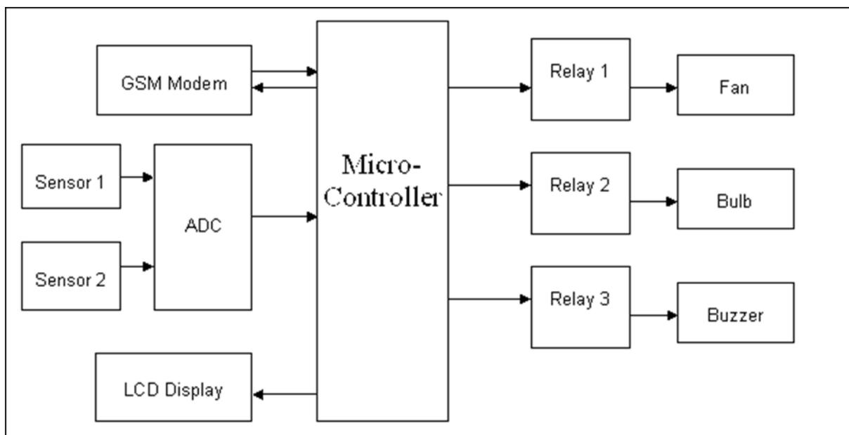
Fig. 1 Block diagram of home automation using GSM
