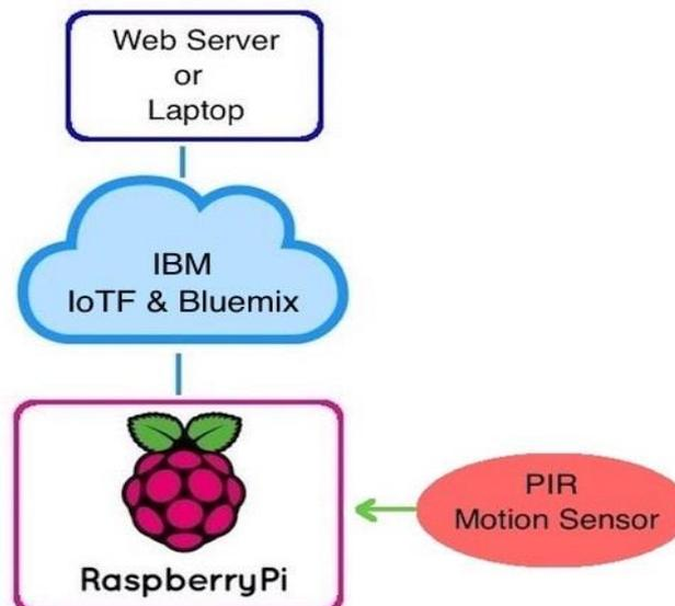
Fig 06: Receiving data from Raspberry Pi
