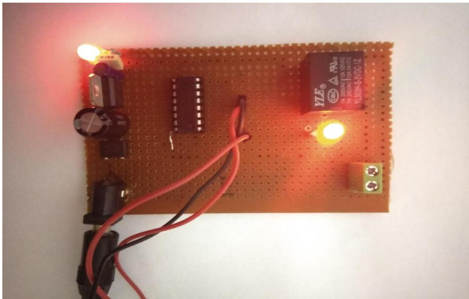
After giving the “light on” command, the LED on the PCB turns on as shown above.
