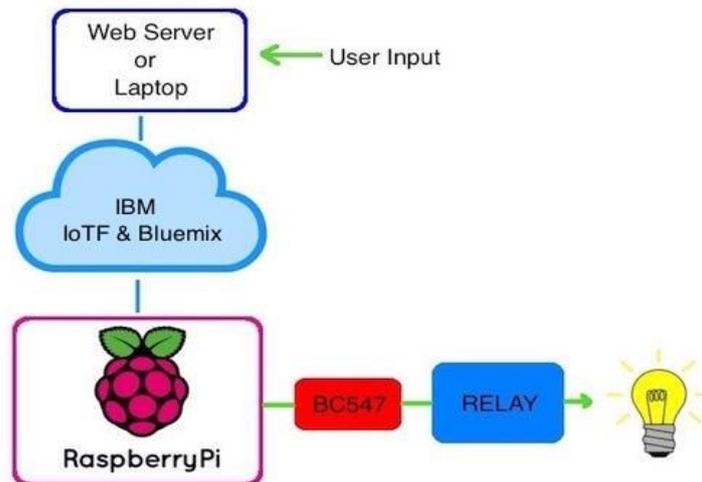
Fig 05: Sending commands to Raspberry Pi
