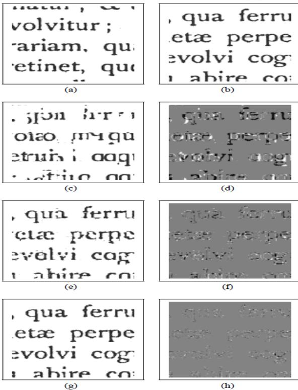
Fig. 3 Approximate pattern matching using inter frame prediction: (a) reference text; (b) current text; (c) predicted text (block size: 16 × 16 pixels); (d) prediction residue (block size: 16 × 16 pixels); (e) predicted text (block size: 8 × 8 pixels); (f) prediction residue (block size: 8 × 8 pixels); (g) predicted text (block size: 4 × 4 pixels); and (h) prediction residue (block size: 4 × 4 pixels) [Adapted from (4)].
