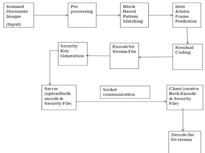
Fig. 2 The block diagram of the H.264 video codec (proposed scheme)
