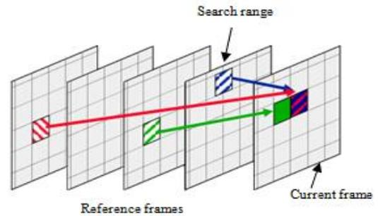
Fig. 4 Block-based motion estimation
