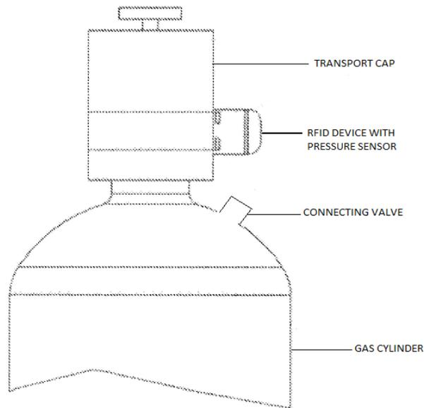
Fig.1.Gas cylinder with RFID Device
