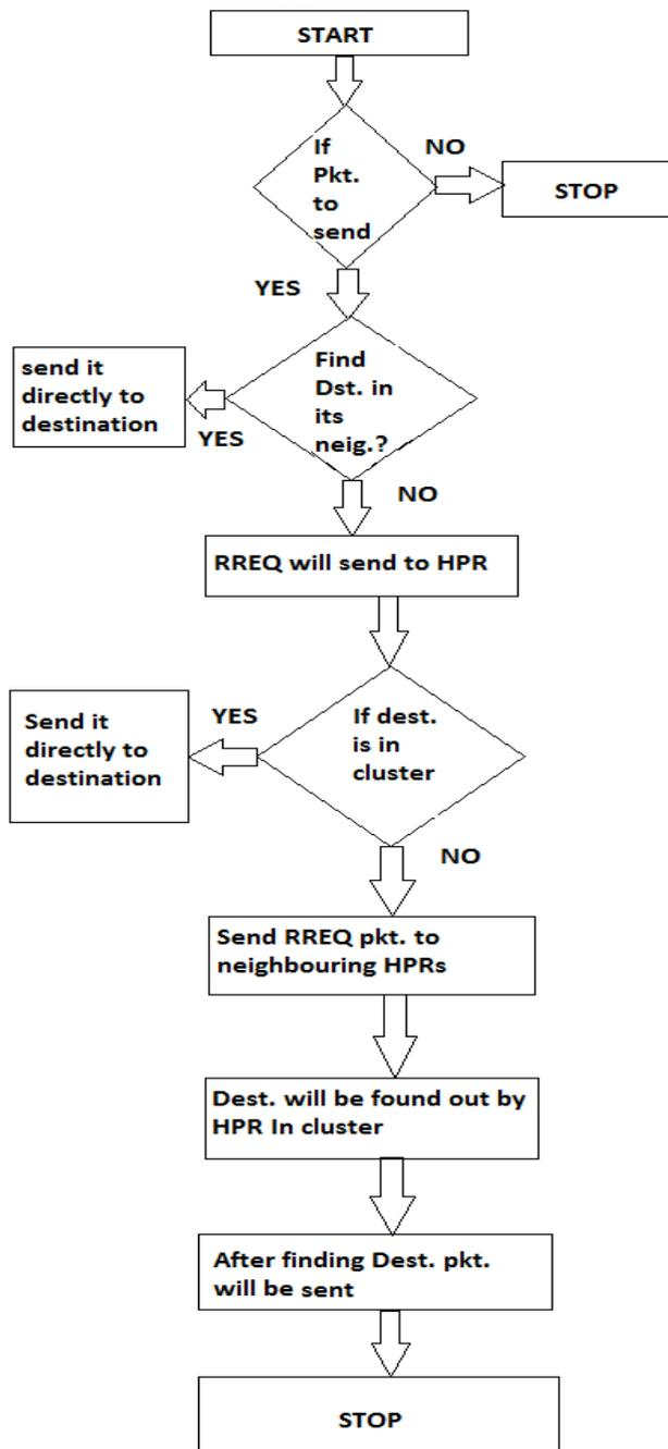
Figure 3. Flowchart of propose system
