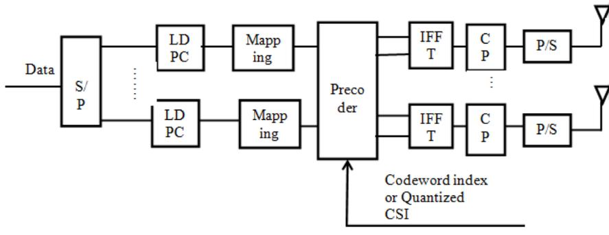
Fig. 1 MIMO – OFDM Transmitter with Precoder
