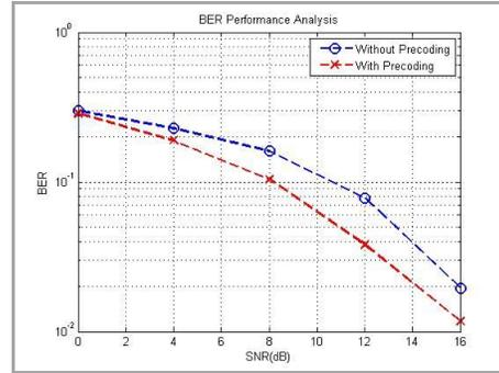
Fig.6 BER Performance of 16 QAM with & without precoding
