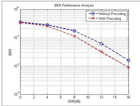
Fig.3 BER Performance of BPSK with & without precoding
