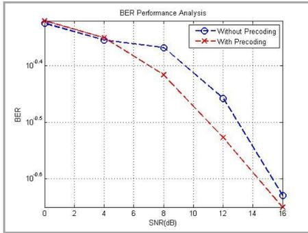
Fig.5 BER Performance of 16 PSK with & without precoding
