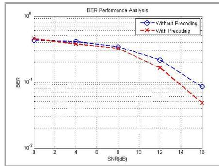
Fig.4 BER Performance of QPSK with & without precoding
