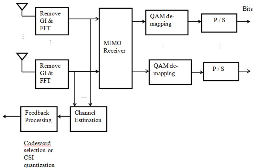
Fig. 2 MIMO – OFDM Receiver with Channel Estimation
